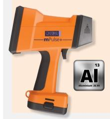
For ultra-fast sorting of a wide range of metal alloys including Magnesium and Aluminium alloys, stainless steels, Ni, Cu, Co, Ti alloys and many more, choose **m**Pulse+.
